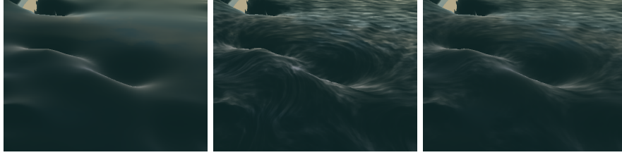
Figure 2.2: The shallow water simulation from Chentanez and Müller renders vortices visible with the addition of high frequency FFT waves and texture coordinates that are advected with the velocity field [CM10].
